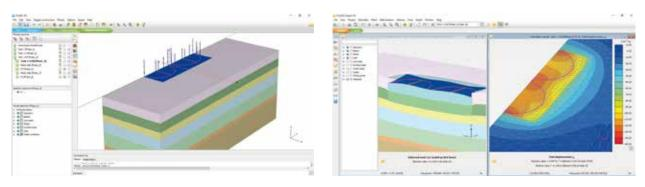
3D Finite element analysis to study the behaviour of two tank foundation
