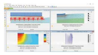
2D Finite element analysis for de evaluation of setlements and soil stresses
