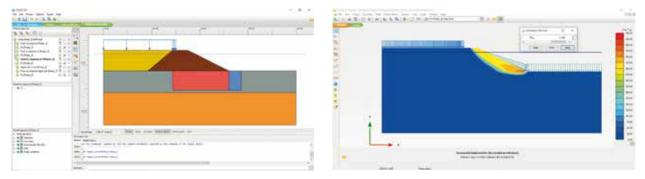
2D Finite element analysis for de evaluation of slope stability in embankments with soil improvement
